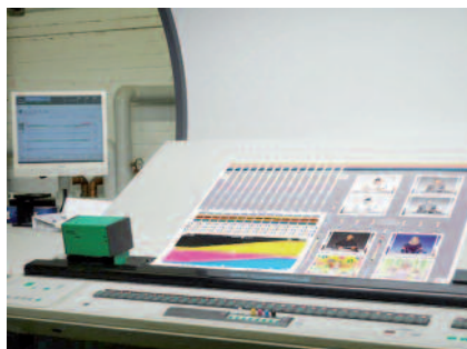
Equipment required includes image analyser to control dot size on plate, densitometer, spectrophotometer, and software for control and visualisation. Source: Sun Chemical
