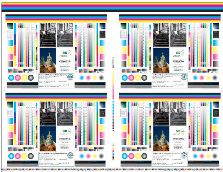
SID test form for certification print (4 times SID test layout on 70 x 100 cm sheet). Source: Hammesfahr
