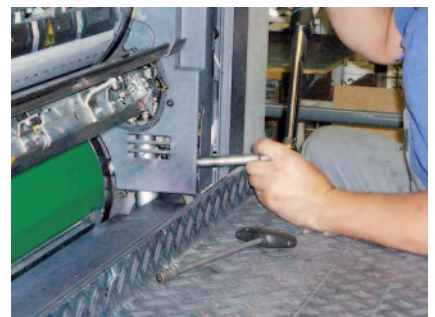
Check blanket packing and tension to ensure printing quality. Photo: GMG
